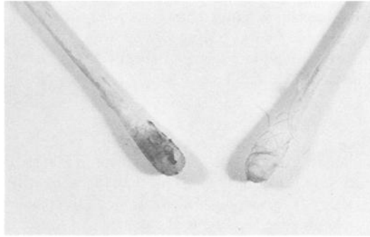
FIG. 8—Positive rhodizonate reaction for lead with control swab on the right. Positive swab from .38 semi-wadcutter solid lead bullet wound.
